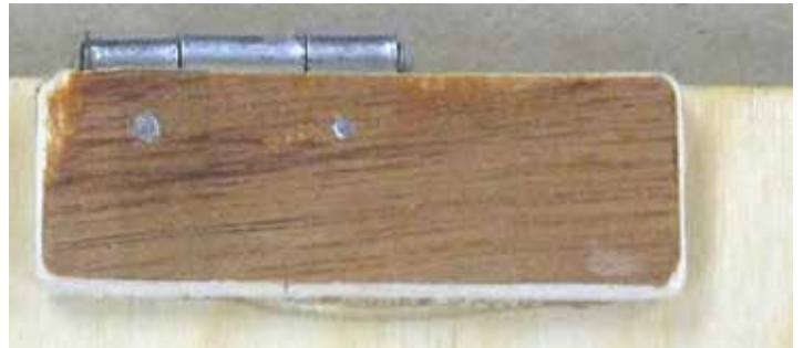
the tips of the screws may be "proud" - file them down if needed
