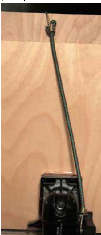
paint panel secured via bungie cord
