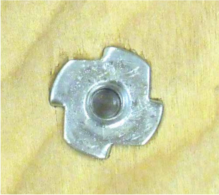
hole drilled and T-nut inserted
